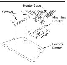
Figure 14 - Cutting Brackets
